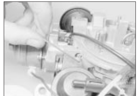
15.9b Choke pull-down adjusting screw
