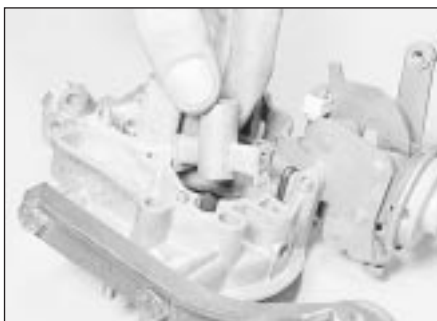
19.16 Removing the pre-atomiser
