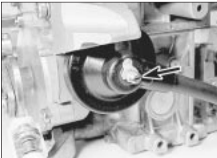
14.8a Choke valve gap adjustment screw (arrowed)
